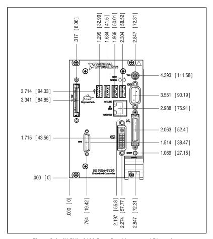
Figure 3-1. NI PXIe-8130 Front Panel Layout and Dimensions
